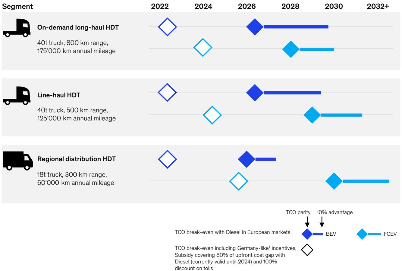
Note: TCO model assumes the following cost levels for HDT long-haul line-haul truck in Europe in 2030: Upfront vehicle costs: 110k USD (ICE)/170k USD (BEV)/180k USD (FCEV); diesel price: 1.20 USD/l, electricity price: 0.13 USD/kWh, hydrogen price: 4.4 USD/kWh. Due to intense truck use, TCO is highly sensitive to energy prices
